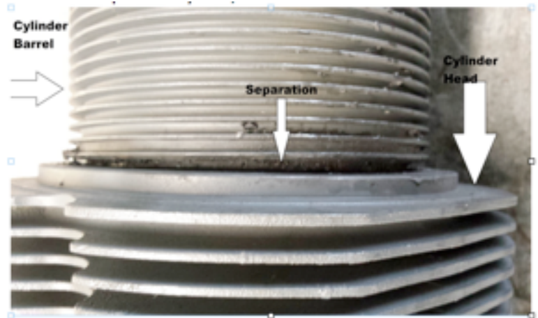
N67818's faulty cylinder
