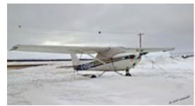
Before delving into a wide range of topics, he stressed the importance of always connecting the power cord to the oil pan heater when the planes are tied down. The oil congeals at low temperatures putting a strain not only on the battery but also on the engine itself. This important fact was later echoed by Dan Coles who elaborated on this issue.
