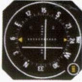
1. Continuing the maneuver on page 77, APPR coupling occurs ("APR" light comes on steady, "HDG" light goes off). The autopilot will roll the aircraft out on localizer and the course index will center.
